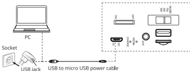
Fig. 2. Connection diagram
