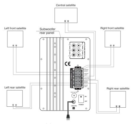
Fig. 3. Speakers connection diagram
