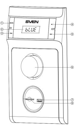
Fig. 1. Subwoofer control panel
