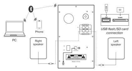
Fig. 5. Bluetooth module connection diagram
