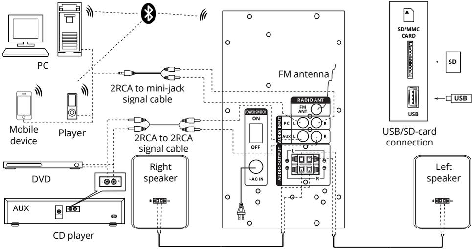
Fig. 5. Connection diagram
