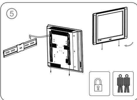
• Fix the mount on the wall using dowels (see Fig. ③).
