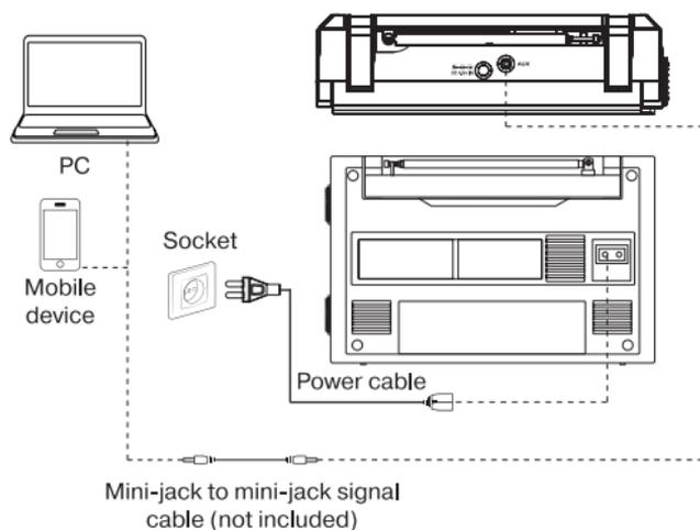
Fig. 3. Connection diagram
