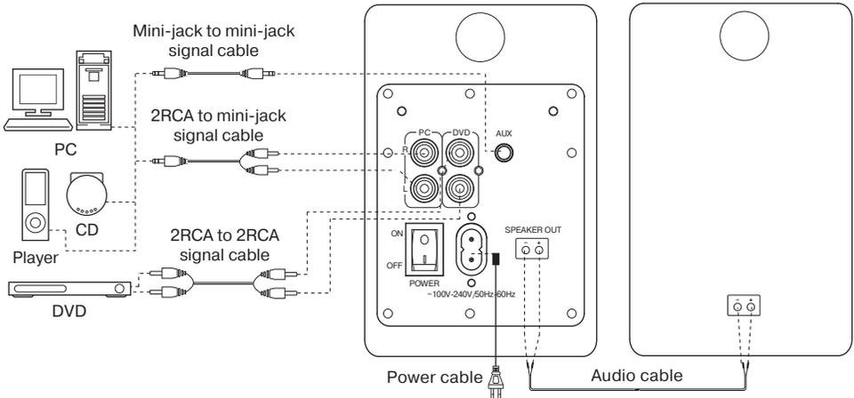
Fig. 4. Connection diagram
