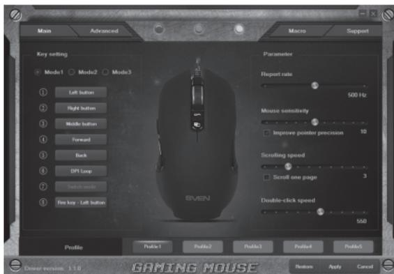
Initially, all mouse buttons are set to their default settings. However, the user can change the keys functions. The only key that can not be reassigned is the key with the number 7 "Switch mode" (not active, highlighted in gray), switching modes "Mode1", "Mode2", "Mode3". You can reassign the buttons by clicking on the menu items, thus pop-up menu, in which you can redefine the keys, assign a macro (pre-configured shortcut options), bind buttons to the multimedia button.
