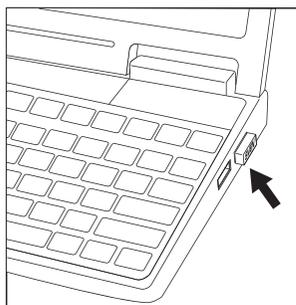
Fig. 3. Receiver connection
