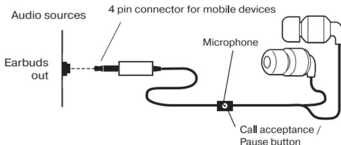
Fig. 1. Connection diagram
